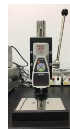
Fig.3 Point load test apparatus
